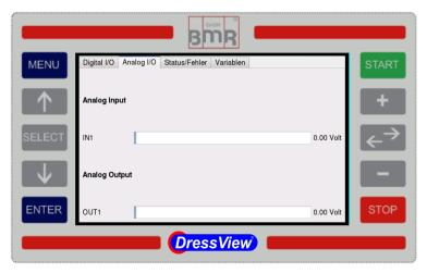
This window displays all analogue I/Os of the converter with it's function and it's current state as bargraph and numerical with it's voltage.
