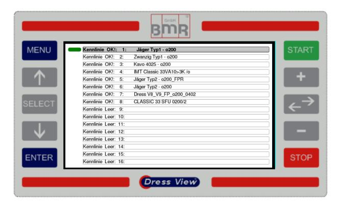
To change the current selected spindle characteristic or list all available characteristics, it has to be moved to the Main-Menu by pressing **MENU**. Being there, it has to be navigated with the **SELECT** or **Arrow Keys** to the point "**Characteristic Selection**" and confirmed with **ENTER**.
