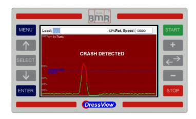
This value can be adjusted in the range from 0 to 100% of the measure value This function is not activated at once with moving to the dressing window (see 2.4.1.9), but only after having carried out a calibration (see 2.4.2.1).
