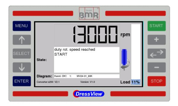
The Terminal-Menu is the window where all basic functions of the converter can be controlled. With the Keys "START", "STOP", "+", "-" and "double arrow" it is possible, to start and stop the spindle and to set up it's rotational speed. Furthermore the current status messages of the converter are displayed, such as selected characteristic, direction of rotation and load status. If an error appears it will displayed in the status area, whose background then turn red.
