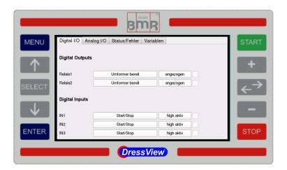
This window displays all digital I/Os of the converter, with it's function and it's current state.
