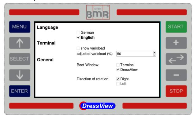
In this window all basic settings can be made, such as system language and the setup and display of the Vario-load function of the converter and the Boot window.
