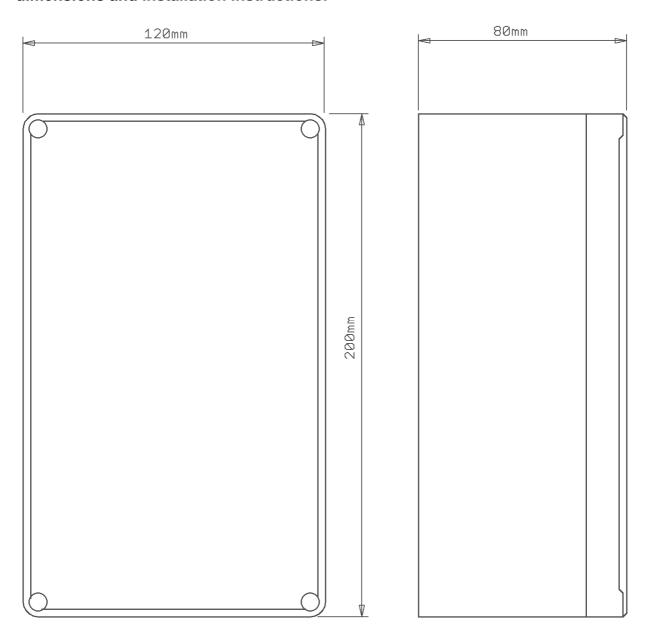
According to standard a retaining clip for C-rail mounting according to standard is located on the back. As an option, mounting bracket for wall mounting are available. There are 4 pieces required and bolted to the back.
