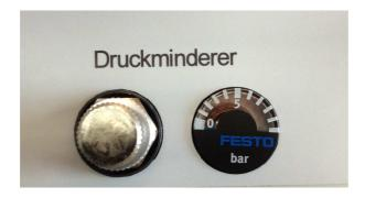
As soon as the outlet pressure is below 0.5 bar, an error is signaled.
